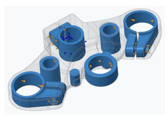
Easily set up optimization by defining the design space, physics, loads and constraint goals, manufacturing process and materials.
